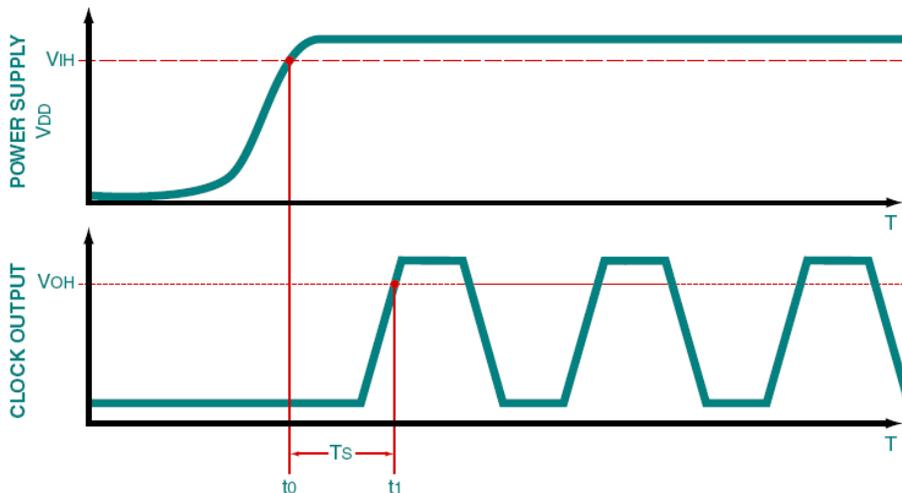
Note: In order to ensure proper start-up, the power supply start-up should have an exponential curve typical of a capacitive charge of a linear voltage ramp. If you have a special voltage start-up profile (i.e. odd ramp steps or shapes), [please contact Ecliptek](#) to discuss possible oscillator performance issues. The maximum start-up time specification for these series can be found on the series datasheet.
