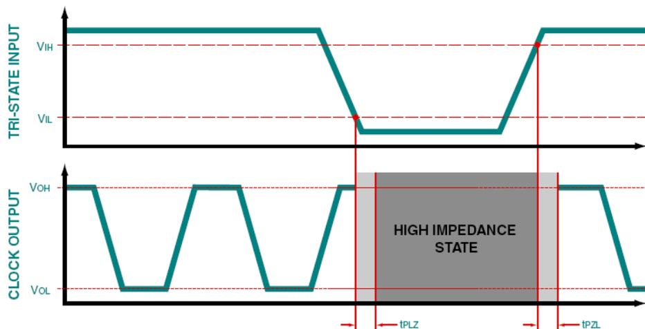
**Figure: Tri-State Timing Diagram**
