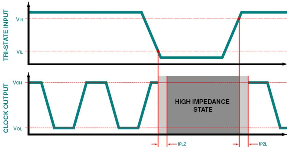
**Figure: Tri-State Timing Diagram**
