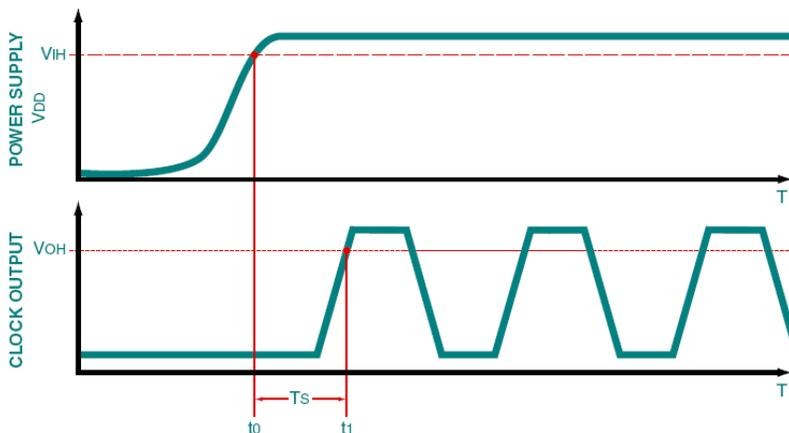
In order to ensure proper start-up, the power supply start-up should have an exponential curve typical of a capacitive charge of a linear voltage ramp. The start-up time specification is listed on the datasheet.
