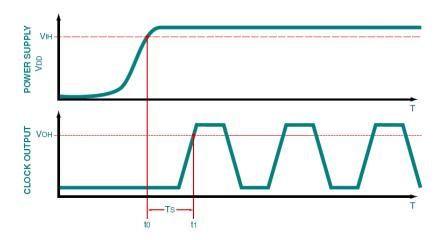
Figure: Oscillator Start-up Timing Diagram
