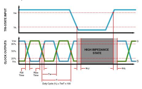
Figure: Tri-State Timing Diagram
