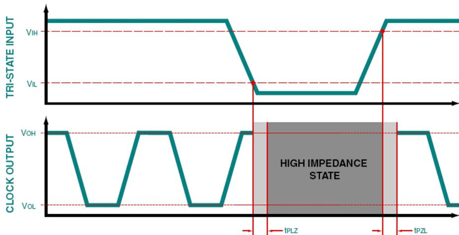
**Figure: Tri-State Timing Diagram**
