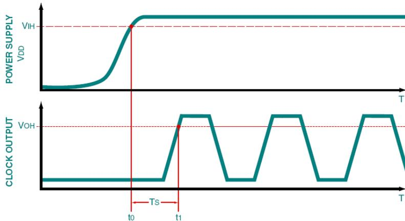
In order to ensure proper start-up, the power supply start-up should have an exponential curve typical of a capacitive charge or a linear voltage ramp. The maximum start-up time specification can be found on the datasheet.
