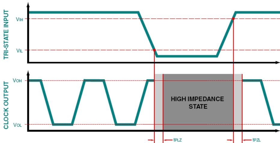
**Figure: Tri-State Timing Diagram**
