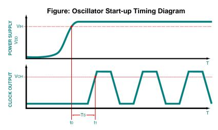
In order to ensure proper start-up, the power supply start-up should have an exponential curve typical of a capacitive charge of a linear voltage ramp. The maximum start-up time specification can be found on the datasheet.
