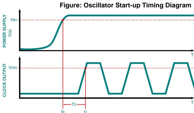
In order to ensure proper start-up, the power supply start-up should have an exponential curve typical of a capacitive charge or a linear voltage ramp. The maximum start-up time specification can be found on the datasheet.
