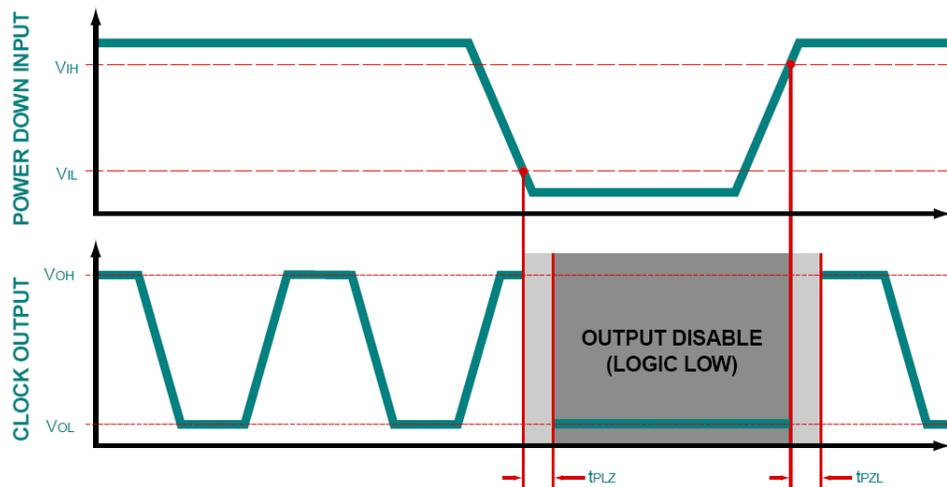
When entering the power down mode, the time from when the oscillator pad one input control reaches  $V_{IL}$  and the oscillator output pad becomes logic low is shown as  $t_{PLZ}$ . When exiting the power down mode, the time from when the oscillator pad one input control reaches  $V_{OH}$  and the oscillator output begins clocking is shown as  $t_{PZL}$ . The oscillator power down disable ( $t_{PLZ}$ ) and enable time ( $t_{PZL}$ ) specifications are listed on the datasheet.
